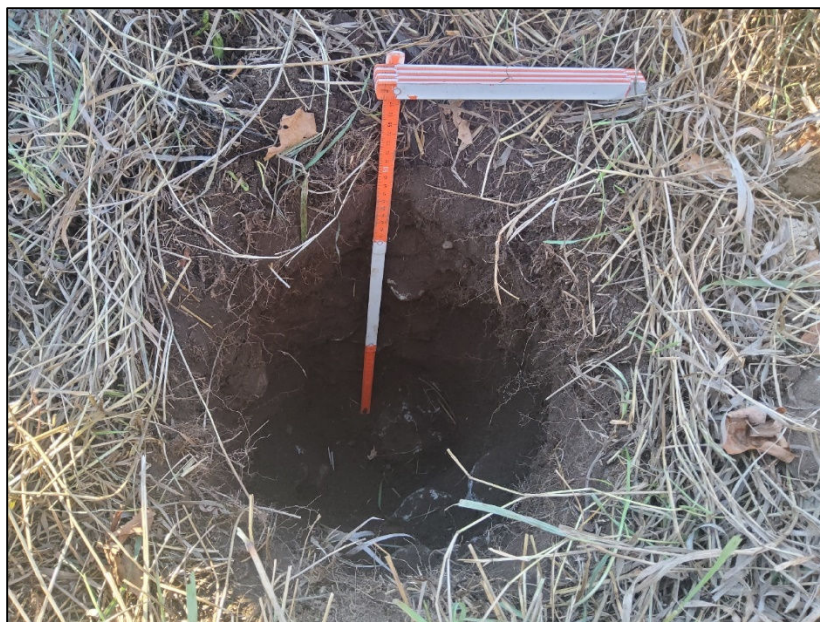
Image 17: View of a disturbed test pit.
