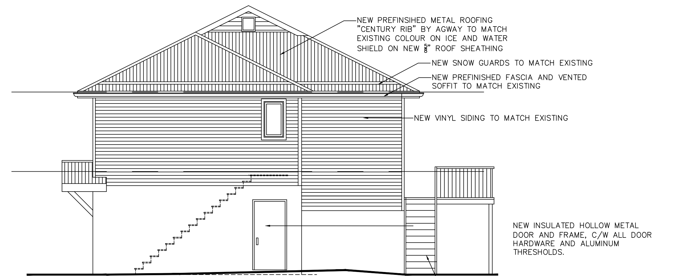
3 EAST ELEVATION SCALE 3/16"=1'-0"
